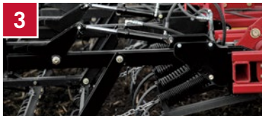
Crumbler pressure: achieve consistent clod sizing and finish
