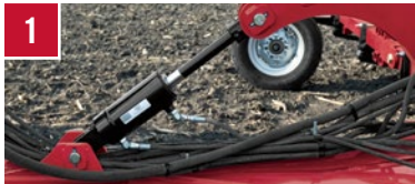
New hydraulic fore/aft control (Constant Level only): maintain consistent agronomic output
