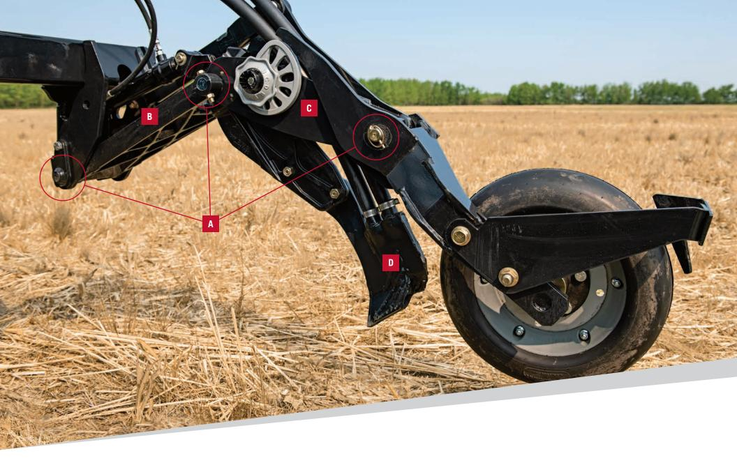
A Sintered metal bushings deliver maximum durability (multiple locations circled)
