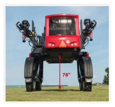
Highest ground clearance on the market! An industry leading 78 inches of ground clearance allows for late-stage application. Easily lower the overall height down to 153 inches (12.75 ft.) from the operator's seat for truck transport.
